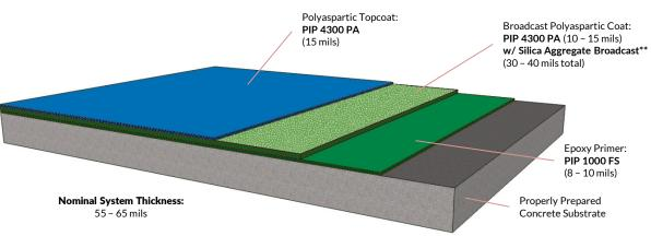
\*\* Broadcast silica aggregate media adds approximately 20-25 mils per broadcast application. \*\* Broadcast silica aggregate at rate of approximately 0.5 to 0.75 lbs. per 1 Sq. Ft.
